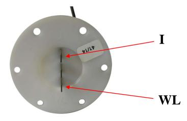
Put the Green/Slate wire to the 'l' terminal (top of gauge) Put the Green/Orange wire to the 'WL' terminal (bottom of gauge) And the black wire to earth
