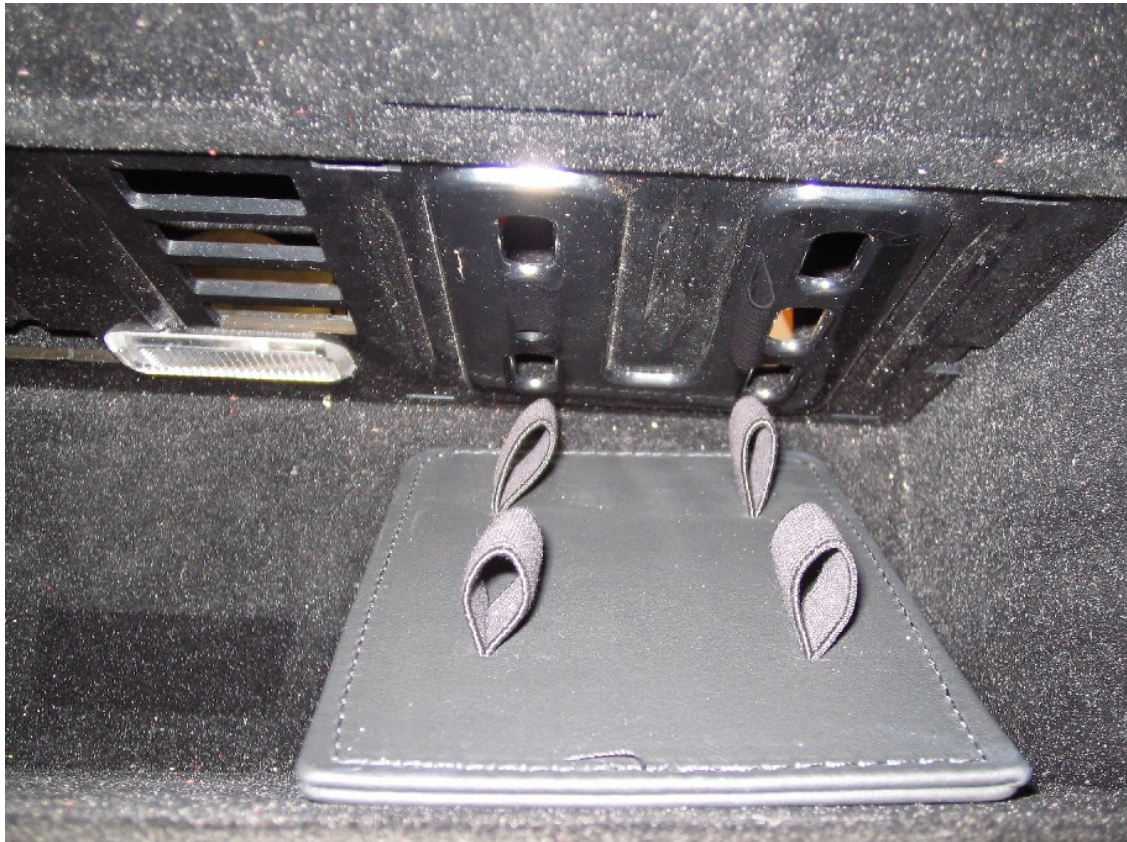
Figure 13a Inserting iPod mounting - post 07MY
