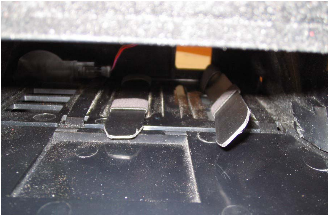
Figure 15 – Install iPod holder to iPod mounting - post 07MY
