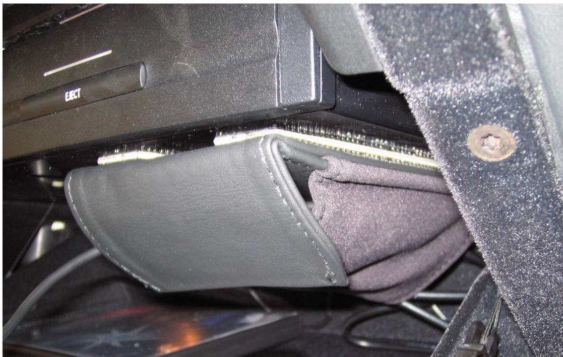
Figure 11 – iPod and USB lead routing through iPod Holder
