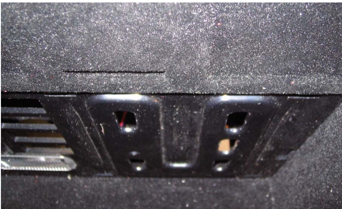
Figure 13 – Inserting iPod mounting 1 - post 07MY
