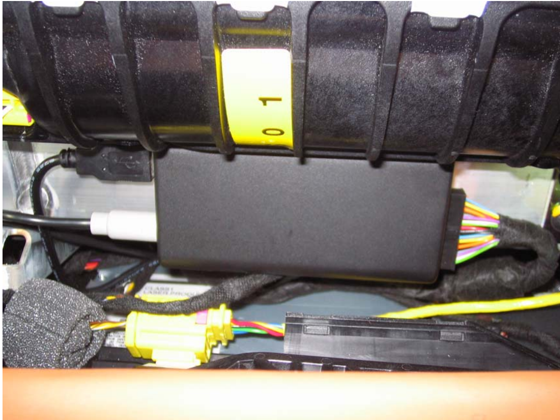
Figure 9 – Installing Pre 07MY Dual Lock strips
