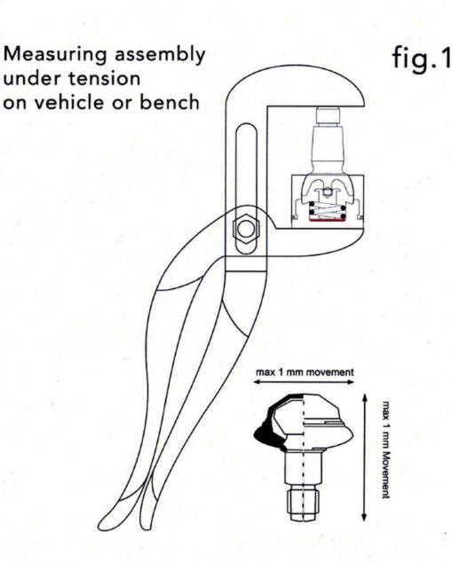
Figures of 1mm 0.040 Inch are established from Drawing RF7552 working specs
