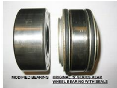
Fig 2 - A new modified bearing and an original S type bearing including oil seals
