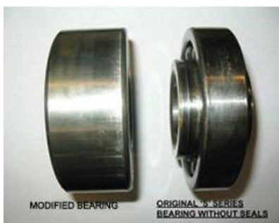
Fig 3 - A new modified bearing and an original S type bearing without oil seals.
