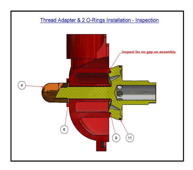
If this operation cannot be implemented by hand without the use of a spanner or socket, it is possible that there is damage to the 1/2"-20 UNF thread within the Domed Nut. Remove all components and inspect. This thread must be in good condition to accept the high torque load applied during installation. If there is damage, do not fit this adaptor. Rectify any damage to the 1/2"-20 UNF thread in the Domed Nut or replace this component. Domed Nut part number is A42994.
