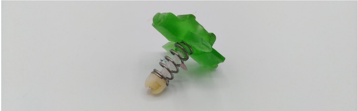
Figure 12: Pin and spring inserted into the toggle. The top is sanded down as described in the previous step
