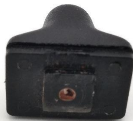
Figure 9: Rocker switch being removed from the switch panel. The bottom is already sanded using 240 and 600 grid paper
