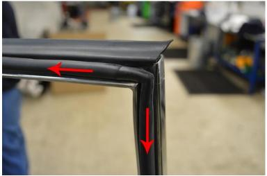
3- Work the seal in to the frame in each direction from this corner until the two ends meet on the underside of the door frame.
